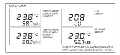
Note: The backlight is permanently on if activated. At 50% intensity the backlight lifetime is approx 10,000 hours. After this time the LCD module needs replacing if the backlight is required. The display continues to operate without the backlight.
