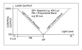
setpoint the loop output is 100%. In the Direct Control mode the output modulates in reverse. The configuration is done via the configuration parameters (or over Modbus).
