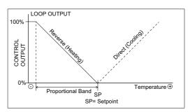
modulate to 100%. When the temperature is the amount of the Proportional Band below the setpoint the loop output is 100%. In the Direct Control mode the output modulates in reverse. The configuration is done via the configuration parameters (or over Modbus).
