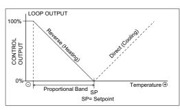
modulate to 100%. When the temperature is the amount of the Proportional Band below the setpoint the loop output is 100%. In the Direct Control mode the output modulates in reverse. The configuration is done via the configuration parameters (or over BACnet network).
