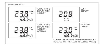
Note: The backlight is permanently on if activated. At 50% intensity the backlight lifetime is approx 10,000 hours. After this time the LCD module needs replacing if backlight is required. The display continues to operate without backlight.
