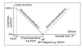
starts to modulate to 100%. When the humidity is the amount of the Proportional Band below the setpoint the loop output is 100%. In the Direct Control mode the output modulates in reverse. The configuration is done via the configuration parameters (or over BACnet network).
