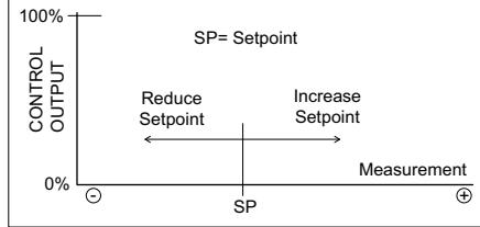
With setpoint options it is possible to adjust the current control setpoint. The setpoint knob option provides rotary knob for the setpoint whereas the SPB option provides two push buttons for setpoint. The adjustment shifts the CO<sub>2</sub>, temperature, or humidity setpoint up or down depending on the configuration parameter settings. The setpoint can also be made only to be
