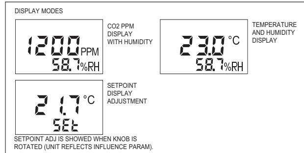
*Note: The backlight is permanently on if activated. At 50% intensity the backlight lifetime is approx 10,000 hours. After this time the LCD module needs replacing if the backlight is required. The display continues to operate without the backlight.*
