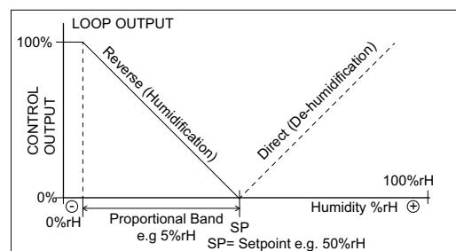
The humidity control loop can also be configured to operate as Proportional + Integral control by changing the Integral Action Time from 0 to a required value.
