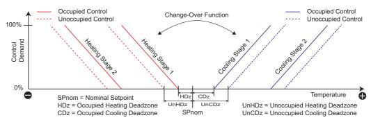
The multi-stage temperature control loop can be configured to control built-in temperature, Universal Input 1 temperature/voltage, Universal Input 2 Temperature/voltage, or network value (network temperature).
