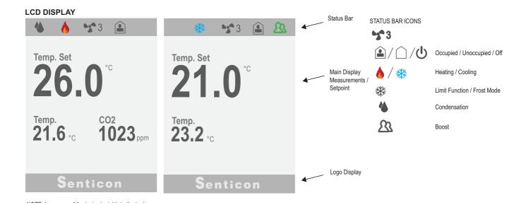
The display has area for controller status indication and main area for the temperature / CO2 and setpoint display. The display main are can be configured to show:-
